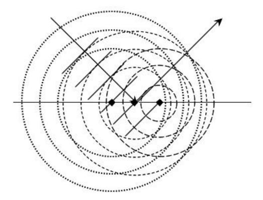
The parallel straight lines indicate maximum positive amplitudes of a wave.
